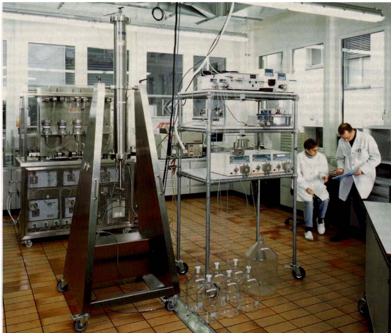
CHIRAL CHROMATOGRAPHY Simulated moving bed installation at CarboGen subsidiary of Solutia, Aarau, Switzerland, separates 4 kg of racemate per day.
