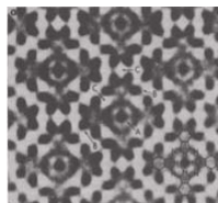
TEM image of F_{16} -CuPC - Electrons are localized in a molecule
