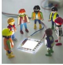
Philips Lighting/Novaled 25 lm/W @ 1000 cd/m 2
