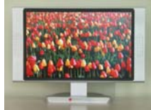
LG전자-LG Philips LCD (2004) 20.1" XGA (1280×800) Poly-Si TFT AMOLED
