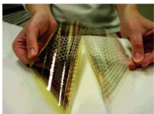
Optical image of 6 in 6 in RFID circuit array (right) fabricated on polymeric substrate, via the polymeric shadow mask shown at left.
