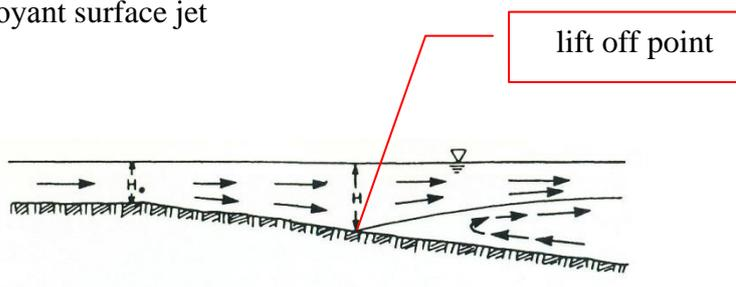
~ is likely to remain attached to the bottom for some distance, and then to spring from the bottom because of buoyancy.
