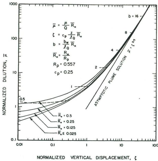
Fig. 2.28 Normalized dilution vs normalized vertical distance
