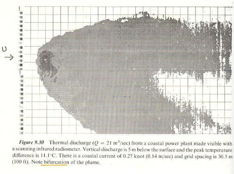
Fig 2.30 Thermal discharge ( $Q = 21 \text{ m}^3 / \text{s}$ ) from a costal power plant
