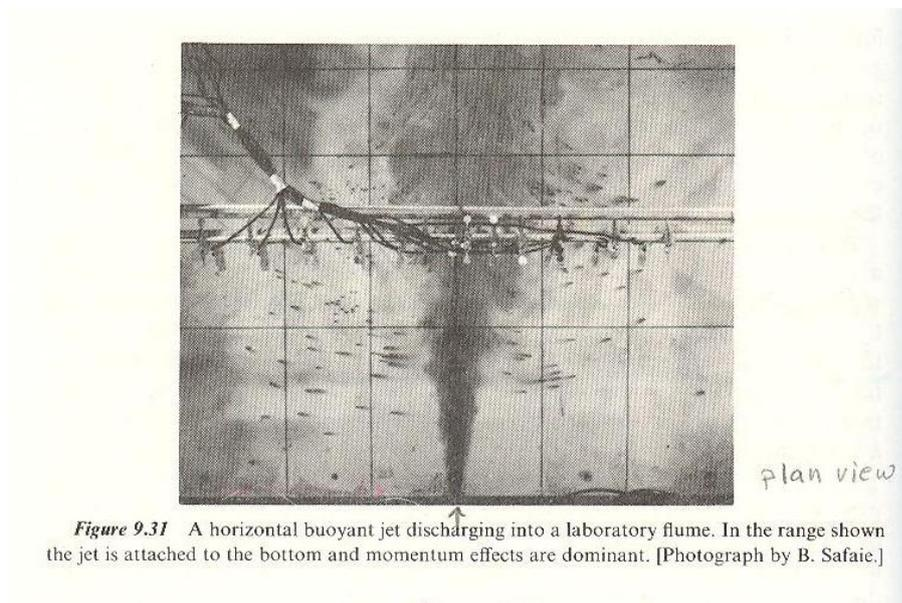
Fig. 2.31 A horizontal buoyant jet discharging into a laboratory flume
