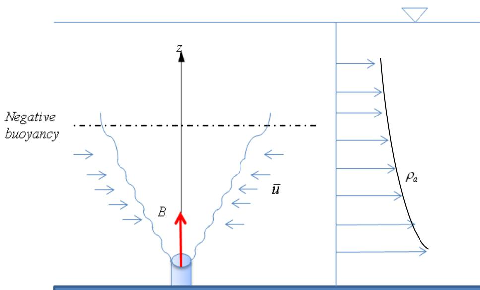
When a turbulent buoyant jet is rising in a density-stratified environment, the fluid entrained at a given level is denser than that at a higher level.
