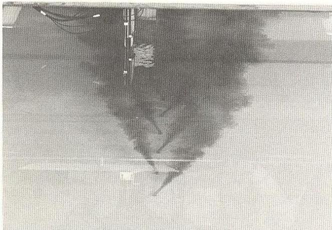
*Figure 9.37* A model section of a multiport diffuser. Each discharge port is angled  $20^\circ$  up from horizontal; ports alternate  $\pm 25^\circ$  from diffuser axis. Model scale 49.3 : 1,  $R_0 = 0.03$ .
