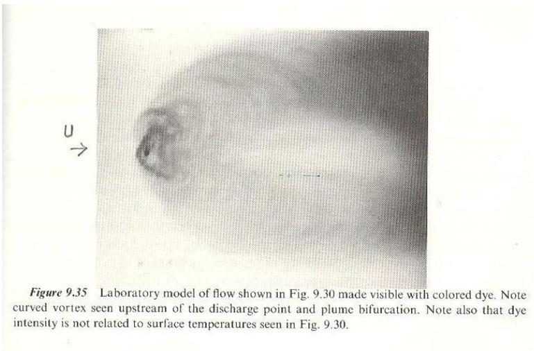
*Figure 9.35* Laboratory model of flow shown in Fig. 9.30 made visible with colored dye. Note curved vortex seen upstream of the discharge point and plume bifurcation. Note also that dye intensity is not related to surface temperatures seen in Fig. 9.30.
