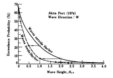
exceedance prob.  $(H_i > \text{ specified } H_i) = \text{exceedance prob.} (H_s > \text{ corresponding } H_s)$ assuming 1 to 1 correspondence between  $H_i$  and  $H_s$  for given wave direction.
