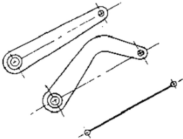
Kinematically identical binary links (two joints)
