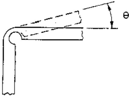
Flexural pair. Used for limited turning.
