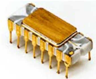
Intel 4004(1971), 4 bit processor, has 2108 transistors
