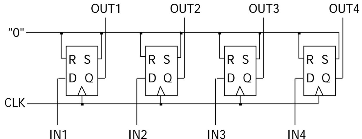
From now on, we will look at a collection of FFs. The first memory element to look at is a register. A register is normally defined as a group of FFs with coordinated controls or shared controls. Examples of controls are clock, reset, set and so on. In this case, we can read/write 4 bits in parallel.
