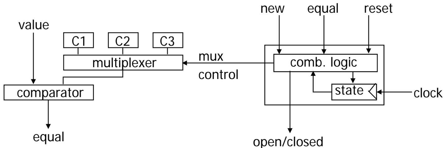
In most sequential logic circuits (SLCs), there are storage parts or memory elements. Recall that in the door lock system, three numbers should be stored and compared. What is the key element here?
