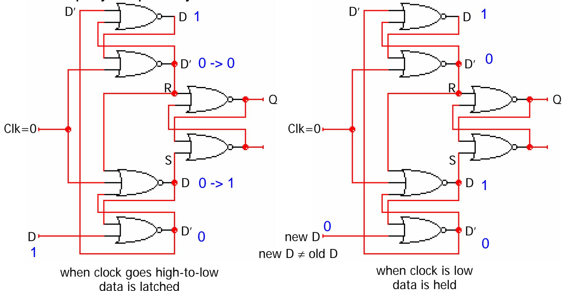
If clock goes from 1 to 0, initially S and R are 0. Then, depending on D's value, S or R will be changed, which in turn will set or reset Q. The numbers in blue shows the case when D is 1. After that, D's change makes no effect. E.g. new D is 0 now, D (second bottom NOR) was 1. D' (bottom) is 0. So D (top) is still 1. R and S are not changed
