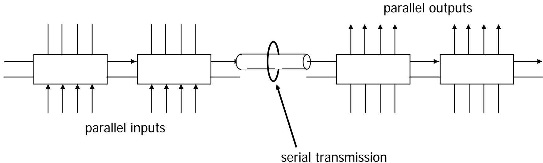
One of the popular application of the shift register is serial transmission, where information is transmitted over the medium bit-by-bit.
