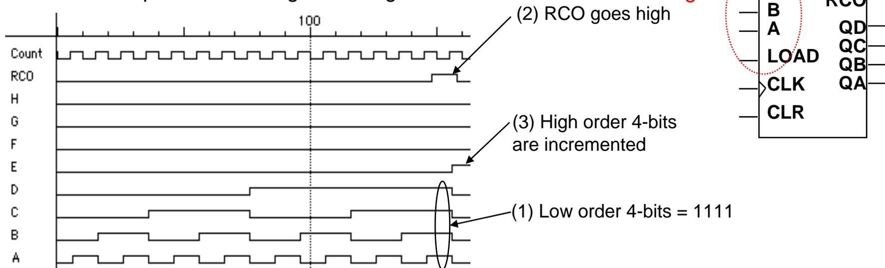
If we use the binary counter in the previous slide as a basic component, we can build many complicated circuits, e.g. a wider binary counter. Here D is the MSB.
