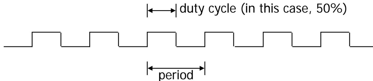
A clock is an important element in sequential circuits. The enable signal in the previous slide serves as kind of a clock. Once enable is asserted, it should remain high until the input stimulates the output fully. Normally, a clock is periodically alternating between high and low. The beginning of each period is called a clock tick. And the duty cycle is defined as the ratio of High voltage interval to the period.
