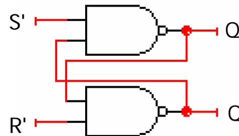
Let's consider this feedback in the cases of cross-connectivity between other gate types. With Nor or Nand gates, we can have more control inputs. R and S denote reset and set inputs, respectively. Q is the output value of interest and its inverse is denoted by Q'. For a NOR gate, think of a case when a single input can determine the output of the gate. Suppose R is 1, which makes Q 0. Basically, we assume R and S are opposite for update.
