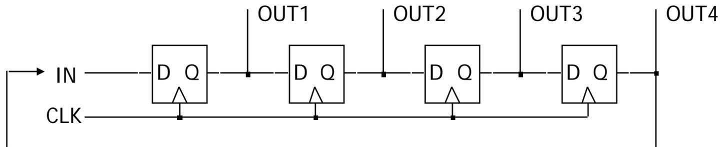
If there are multiple patterns that are used for state representation, this register is typically referred to as a counter. Look at the shift register in the slide. Suppose there is a initialization (or preset) logic that stores 1000 in the register, which is not shown here. Then, as the clock ticks, the bits are rotating this ring. That's why it is called a ring counter.
