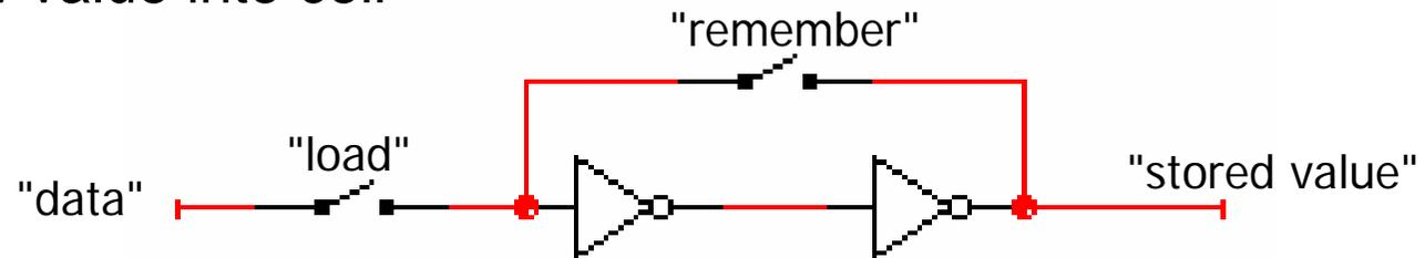
Let's consider a simple memory element first. What if we place two inverters before a stored value and suppose the stored value is 1. Note that there is a feedback from the stored value to the first inverter. Another more sophisticated option is to have a selection function between a stored value and a new value. If "load" is enabled, the new "data" will be put into the stored value.
