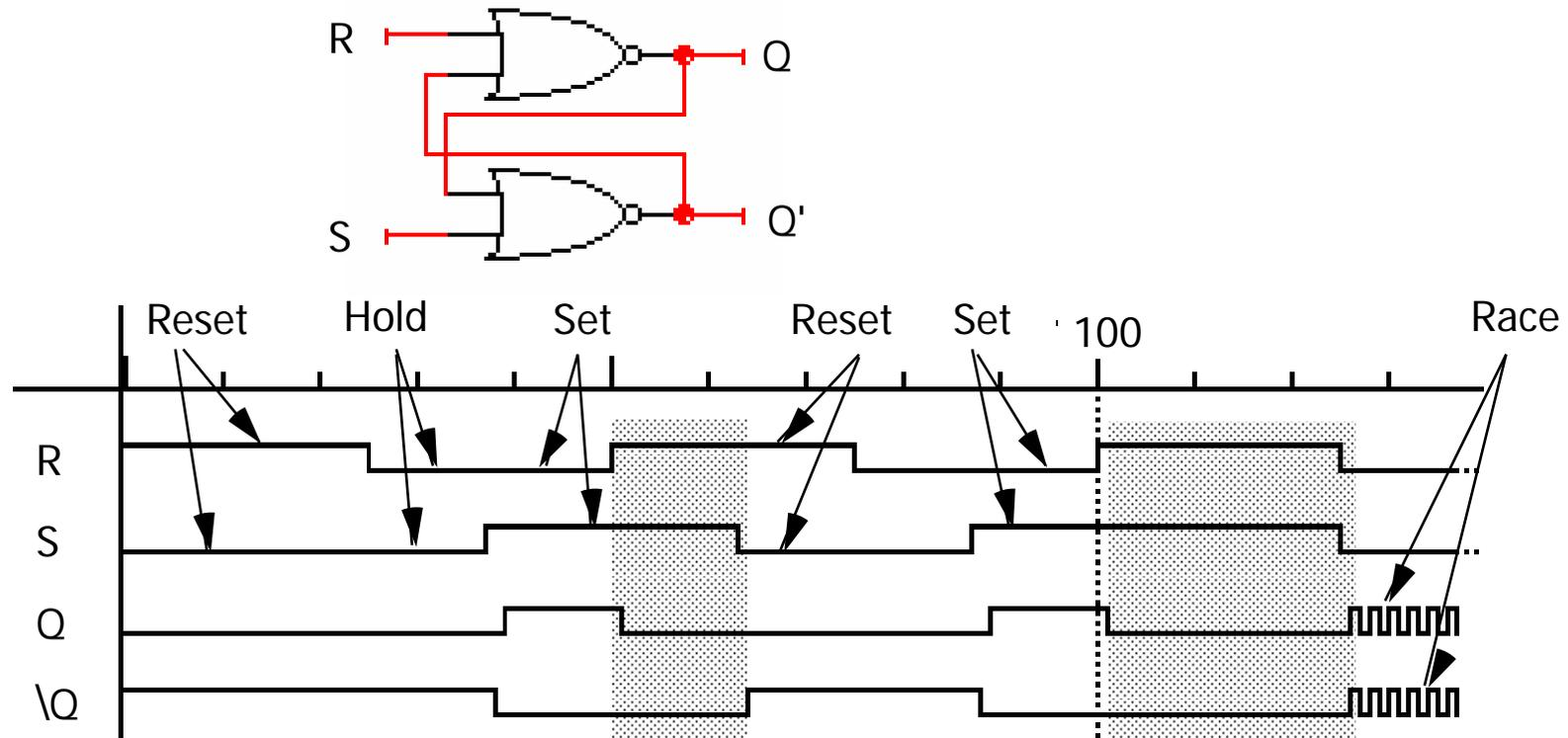
If  $R=1$  and  $S=0$ ,  $Q$  is 0 and  $Q'$  is 1 (recall the meaning of reset  $R$ ). If  $R=0$  and  $S=1$ ,  $Q$  is 1. What if  $R=S=0$ , then  $Q$  and  $Q'$  will remain with the previous values.
