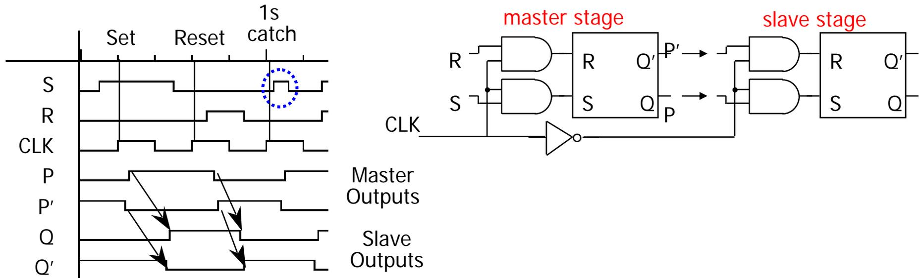
What would be the problem of the inverted clock signals for the pair of R-S latches?
