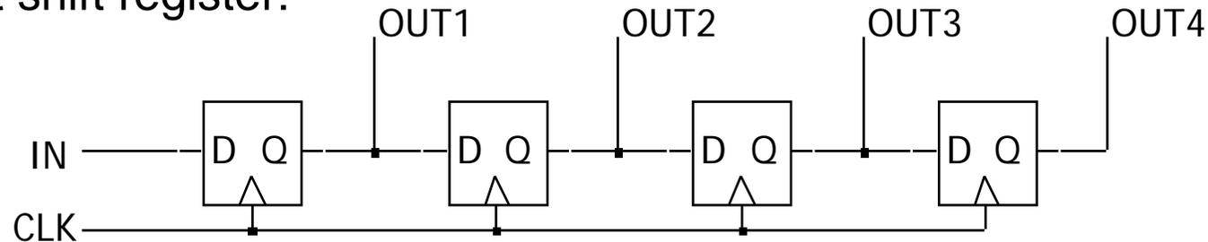
One of the relatively simple registers is a shift register. Here one bit is shifted (or moved to right) to the next FF at each clock tick (its positive edge). At each positive edge, the stored value will come out and move to the next element.
