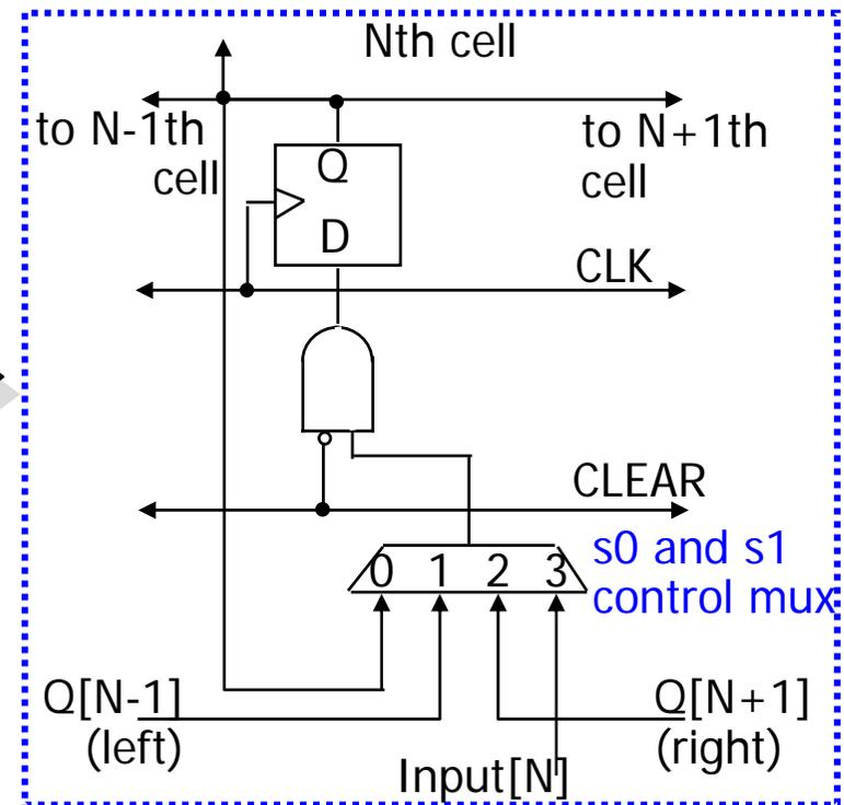
Each memory module (that stores 1 bit) should be able to perform 5 functions. Note that there are multiple incoming lines and one of them should be selected. This should ring the bell. It will be convenient to use a MUX. Blue wires are about control while black wires are data paths. Here, clear, S1 and S0 are depicted by a single wire for simplicity.
