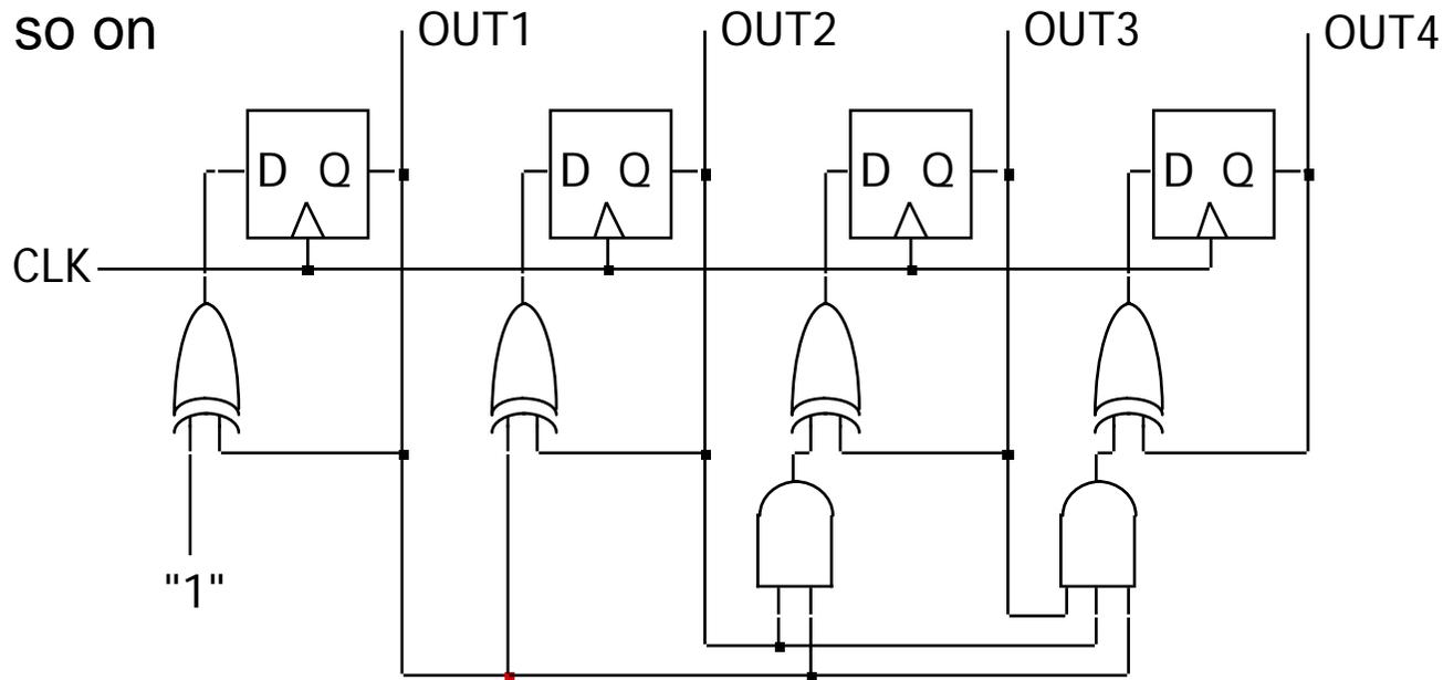
Here is a binary counter; the rule of thumb is that if all lower bits are true, than the upper bit should be toggled. OUT4 is the MSB while OUT1 is the LSB.
