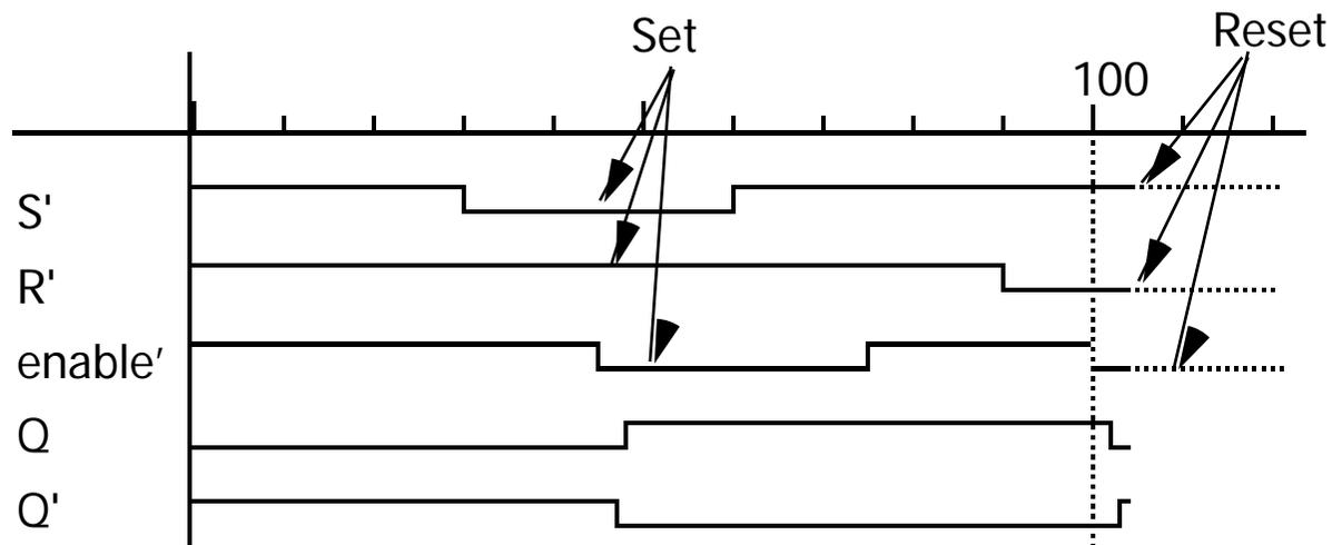
The next version is a gated R-S latch. In the gated (level-sensitive) R-S latch, the R-S values are handled cautiously. When enable' is high, then R and S are always zeroes (there is no glitch or fluctuation in R and S). So R' and S' are meaningful only when enable' is low. This waveform shows when enable is high and S is set (or S' is low), Q will become true.
