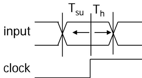
there is a timing "window" around the clocking event during which the input must remain stable and unchanged in order to be recognized
