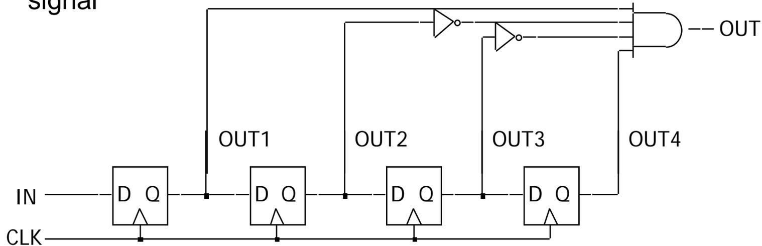
Another useful application of shift registers is bit string identification. In this case, bits are shifted from left to right. At any moment, if 4 bits are 1001, then OUT will be true.
