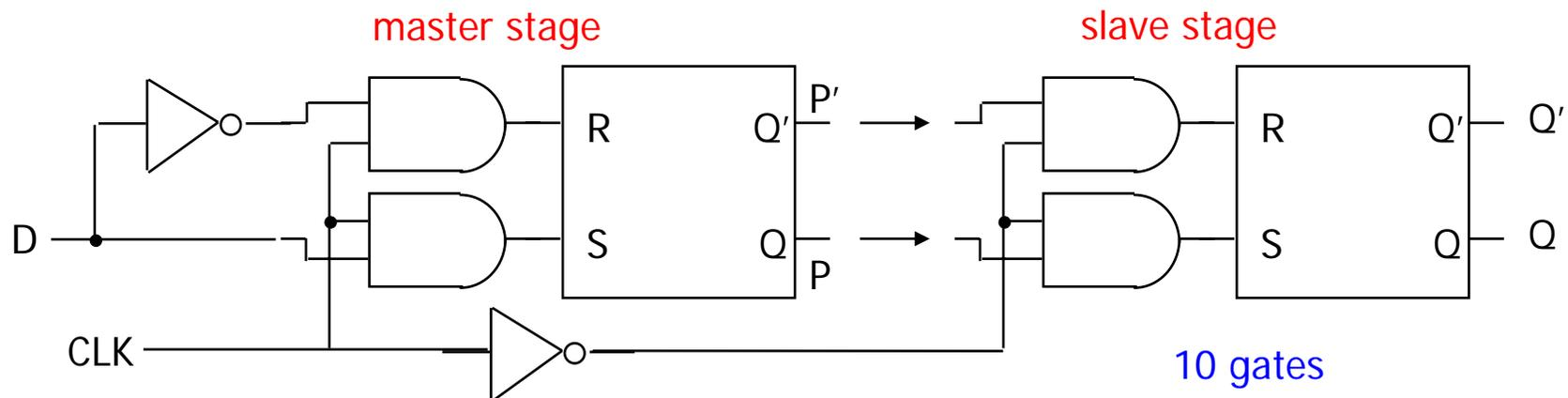
To eliminate the 1s catching problem, we have to make S and R have opposite values; so we use the complementary values from the same input, which is called D flip-flop. D is an abbreviation for data. So R and S can be either 01 and 10 only. Now we cannot use 00 to maintain the same value in the latch. How many gates here? Each R-S latch has two NOR gates.
