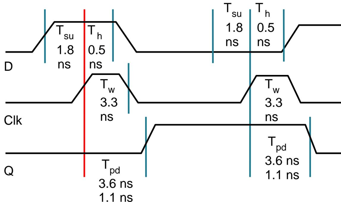
all measurements are made from the clocking event (the rising edge of the clock)
