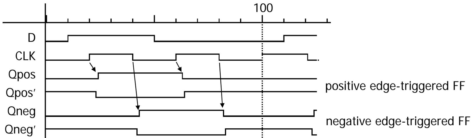
There are two kinds of flip-flops which are triggered by the two edges of the signals: rising edge and falling edge. The previous slide shows a negative edge-triggered FF. If we add an inverter to the clock, that FF is turned into a positive edge-triggered FF. Typically, latches are level triggered and simpler. FFs are mostly edge triggered and more complicated.
