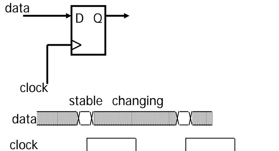
Let's go over terminologies first. We already know what is a clock. For each edge of a clock signal, there are some timing constraints. Suppose the positive edge of a clock signal triggers a circuit. Then the data input should be stable for an interval which is  $T_{su} + T_h$ , which are dependent on transistor circuit delay.
