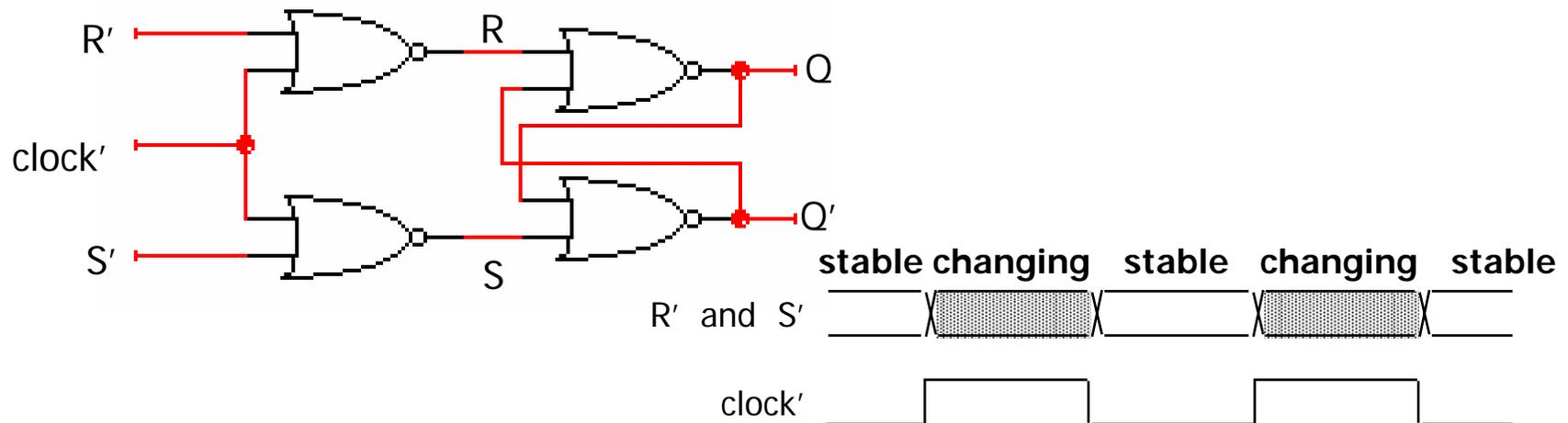
Let's control the gated (or level-sensitive) R-S latch with a clock. While clock' is 0, R' and S' should sustain their values which will update Q and Q' during that interval. While clock' is high, R' and S' can be changed to a new value (for next operation); in the meantime, Q and Q' will not change since R and S are 00.
