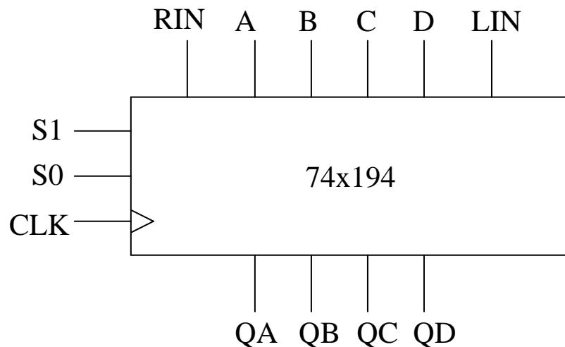
$$DA = \overline{S1} \overline{S0} QA + \overline{S1} S0 RIN + S1 \overline{S0} QB + S1 S0 A$$
