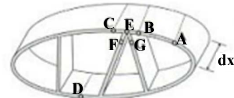
Fig. 8.53 A thin-walled, multi-cellular section under torsion
