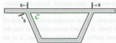
Fig. 8.3. Thin-walled beam with open and closed components.
