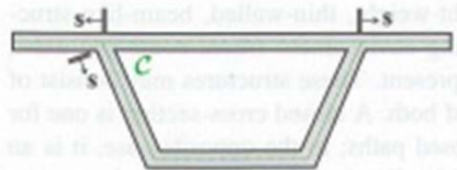
Fig. 8.3. Thin-walled beam with open and closed components.
