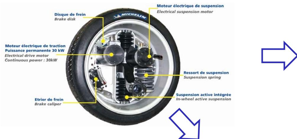
Electric vehicle equipped with Front two in-wheel motors
