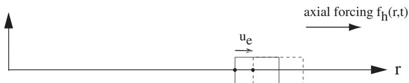
(a) Deformation  $u_e(r,t)$  in axial direction due to axial flexibility
