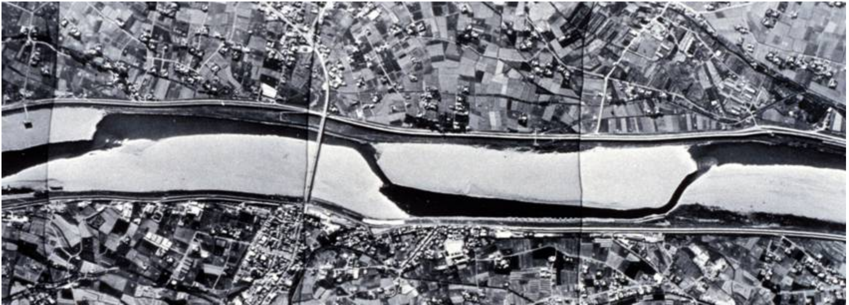
Alternate bars in the Naka River, an artificially straightened river in Japan. Image courtesy S. Ikeda.
