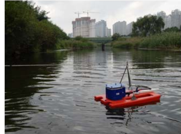
b) Measuring water level using ADCP
