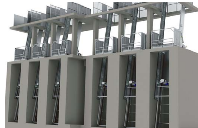
Top: Manually-cleaned bar screen
