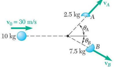
A 10-kg projectile is moving with a velocity of 30 m/s when it explodes into 2.5 and 7.5-kg fragments. Immediately after the explosion, the fragments travel in the directions  $\theta_A = 45^\circ$  and  $\theta_B = 30^\circ$ .
