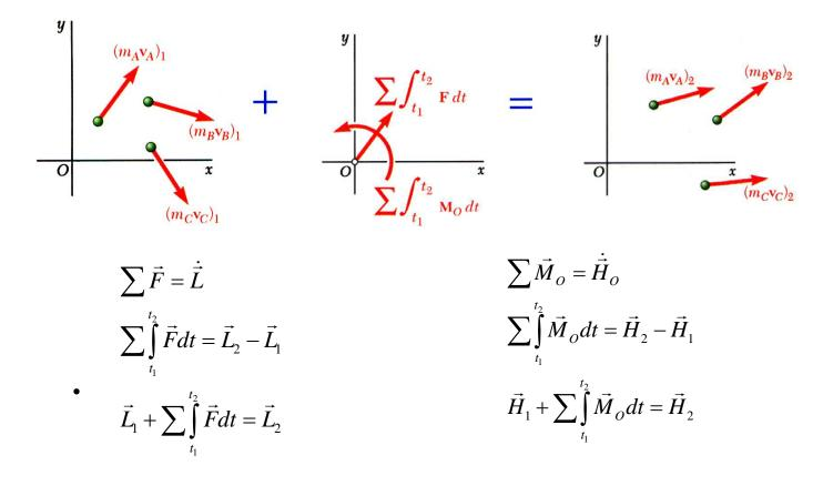
The momenta of the particles at time t<sub>1</sub> and the impulse of the forces from t<sub>1</sub> to t<sub>2</sub> form a system of vectors *equipollent* to the system of momenta of the particles at time t<sub>2</sub>.
