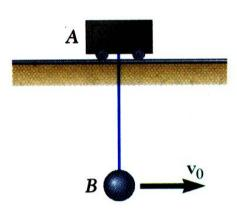
Ball *B*, of mass  $m_B$ , is suspended from a cord, of length *l*, attached to cart *A*, of mass  $m_A$ , which can roll freely on a frictionless horizontal tract. While the cart is at rest, the ball is given an initial velocity
