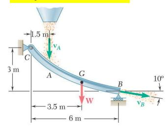
Grain falls onto a chute at the rate of 120 kg/s. It hits the chute with a velocity of 10 m/s and leaves with a velocity of 7.5 m/s. The combined weight of the chute and the grain it carries is 3000 N with the center of gravity at *G*.
