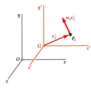
\* Consider the centroidal frame of reference *Gx'y'z'*, which translates with respect to the Newtonian frame *Oxyz*.
