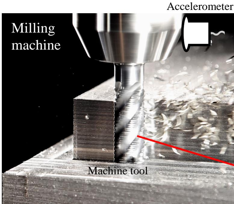
Indirect measurement of wear with vibration
