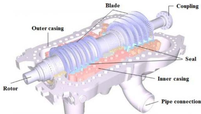
Schematic of a steam turbine
