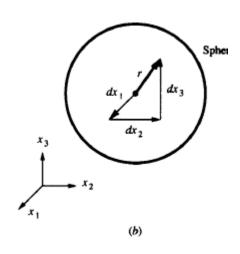
The constraint indicates a circle of radious for 2 dimensions, and a sphere for 3 dimensions
