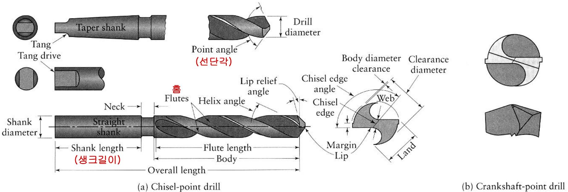
**FIGURE 8.48** (a) Standard chisel-point drill, with various features indicated.
