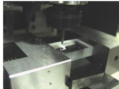
Machining process of 3-axis micro-stage
