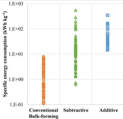
Specific Energy Consumption (SEC) for the three categories of manufacturing process
