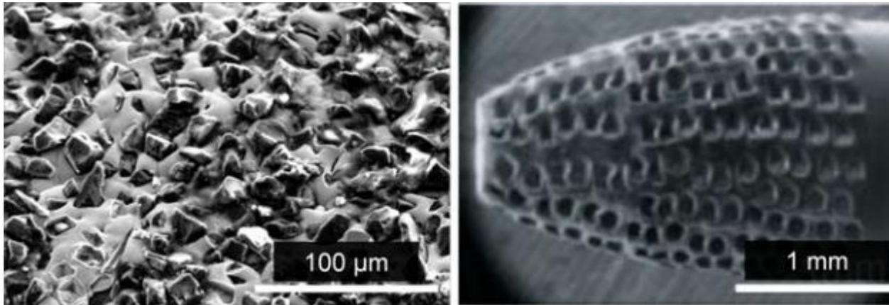
SEM images of the Rotablator burr (left) and a burr with greater-like microblades (right) (Nakao et al. 2005)
