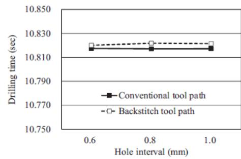
Fig. 11. Drilling time for ten holes.
