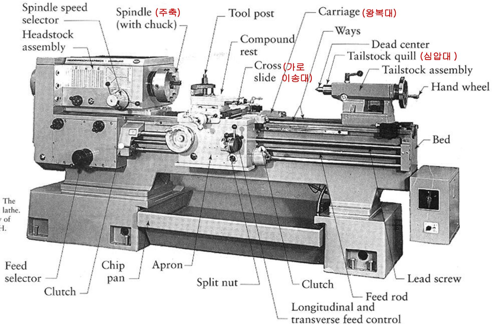
**FIGURE 8.44** The components of a lathe.
