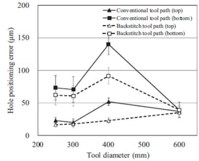
Fig. 6. Effect of the tool diameter on the hole positioning error. The hole interval was twice the tool diameter.
