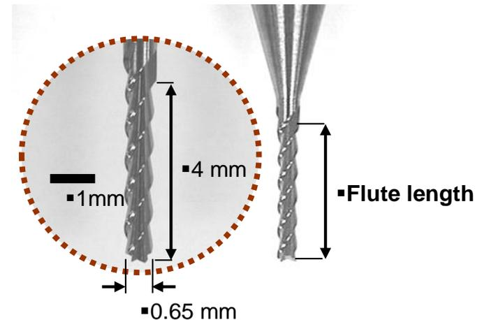
PCB machining micro end mill
