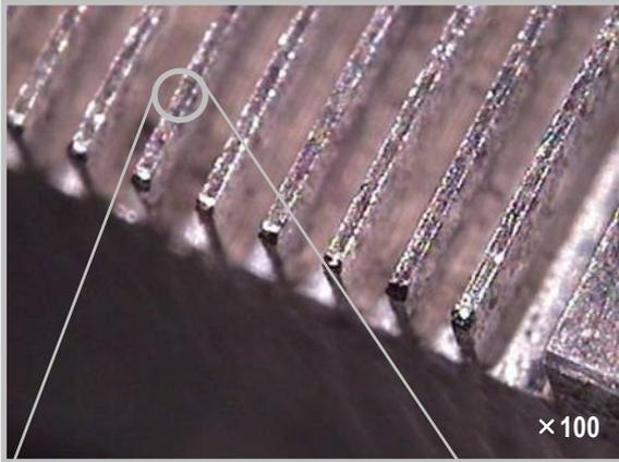
Rib width:  $60\ \mu\text{m}$
