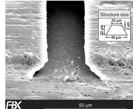
Micro milled undercut-dovetail structure in PMMA.
