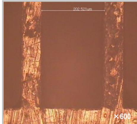
Geometric error:  $\sim 5\ \mu\text{m}$  (including error of microscope)
