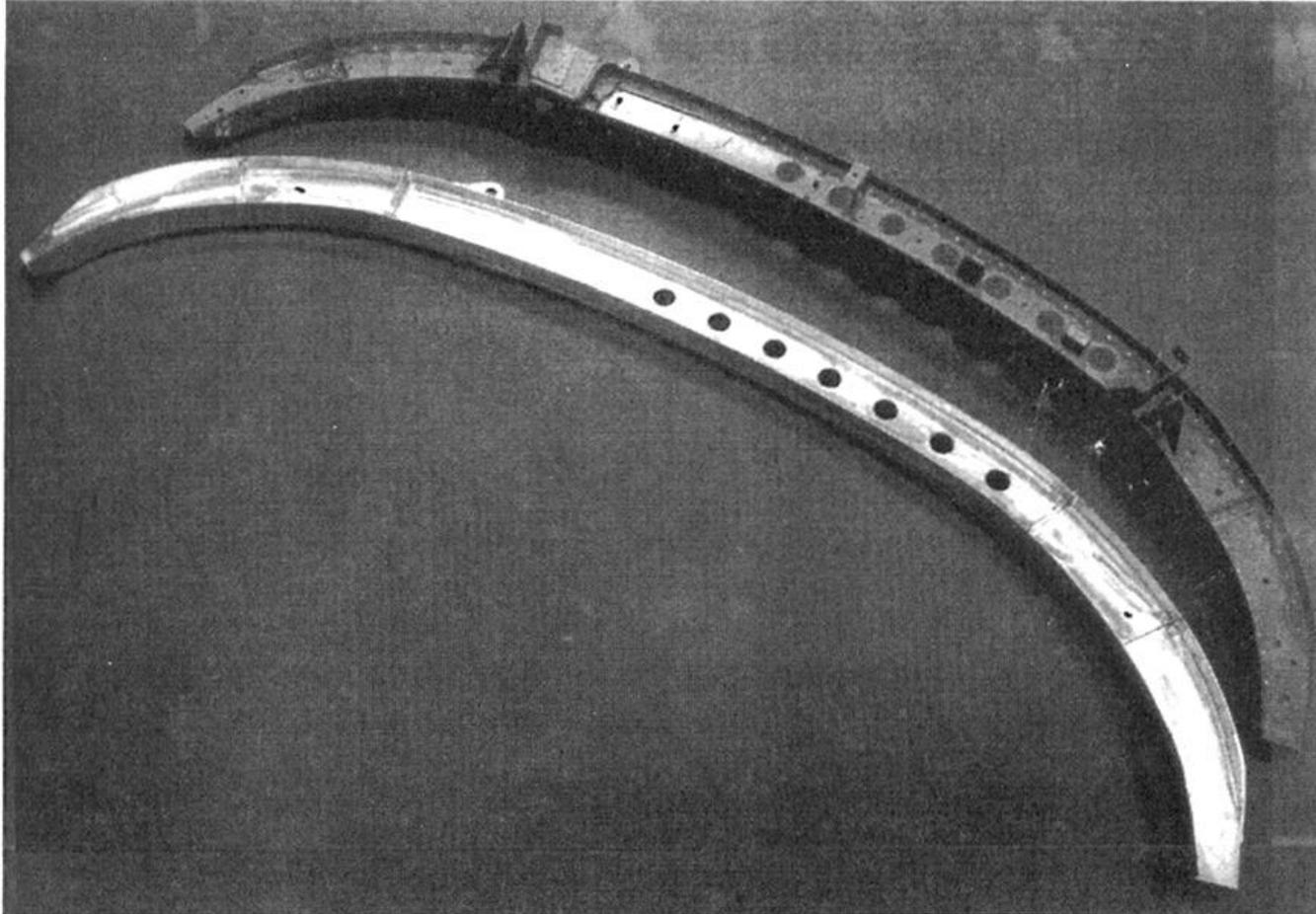
**FIGURE 11.1** Integrated product and process design allows this aerospace component to be completely machined from the solid as shown in the lower photograph (Courtesy of Dr. Donald Sandstrom, The Boeing Company)
