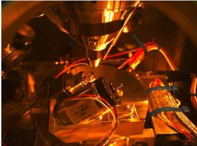
Precision wheel stage attached to the FIB system
