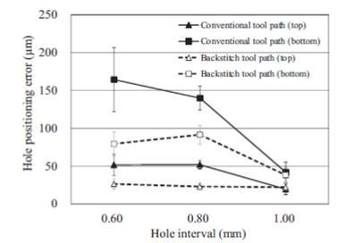
Fig. 8. Effect of the hole interval on the hole positioning error (tool diameter: 400 µm, spindle speed: 90,000 r/min, in-feed rate: 40 mm/s).
