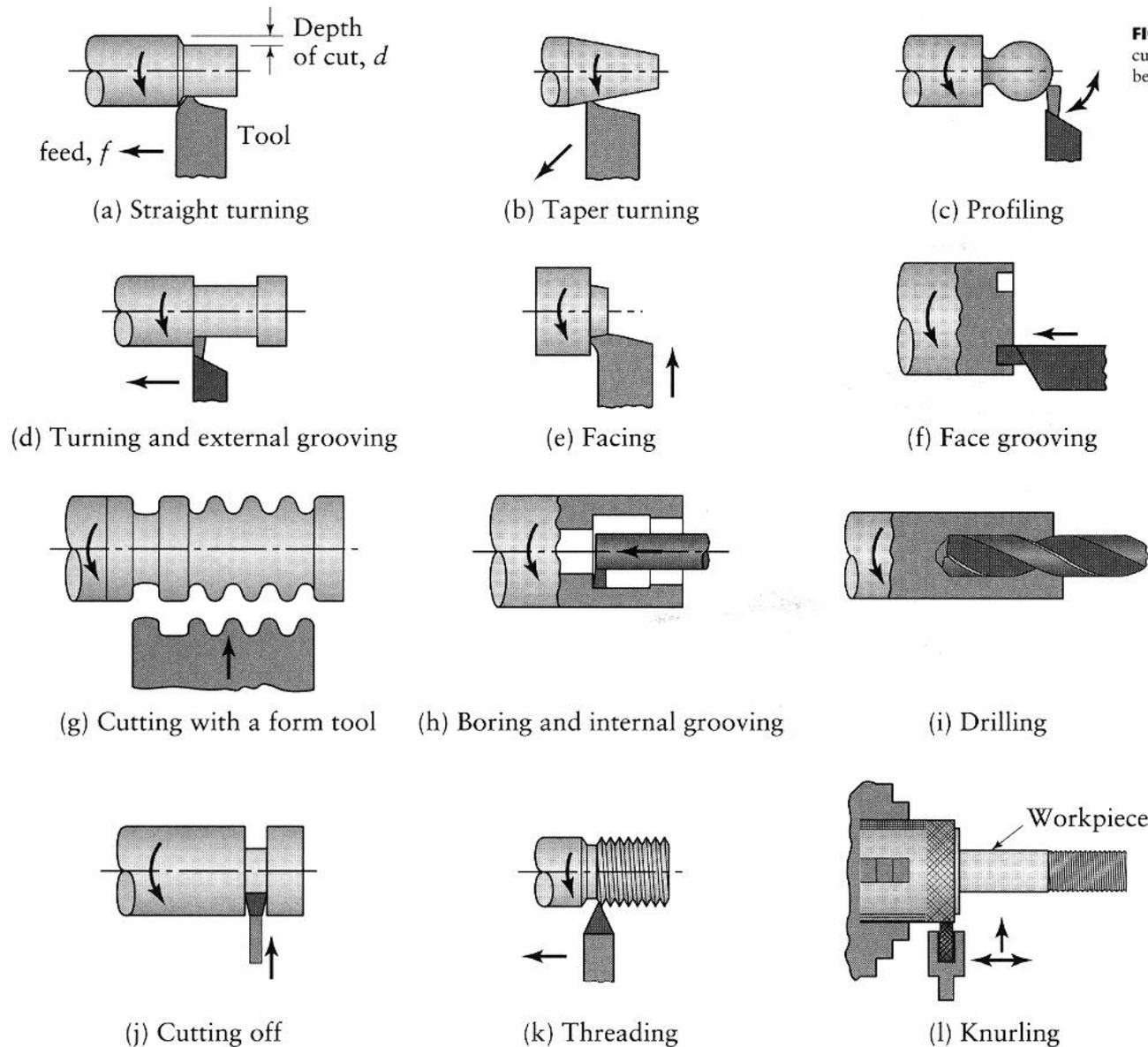
**FIGURE 8.40** Various cutting operations that can be performed on a lathe.
