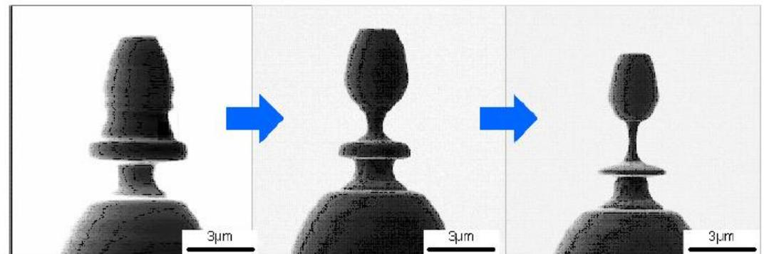
Scanning ion scope image showing the intermediate processing
