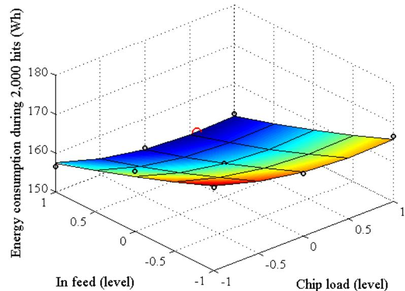
Integrated energy consumption during 0~2,000 holes (**Integral**)
