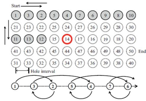
Comparison of the backstitch tool path with a conventional tool path
