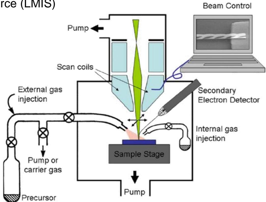
**Schematics of focused ion beam system**
