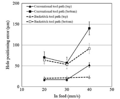
Fig. 9. Effect of the in-feed rate on the hole positioning error (tool diameter: 400 µm, spindle speed: 90,000 r/min).
