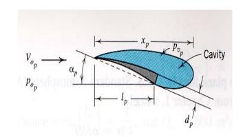
[Ex.1] cavitating hydrofoil model in a water tunnel
