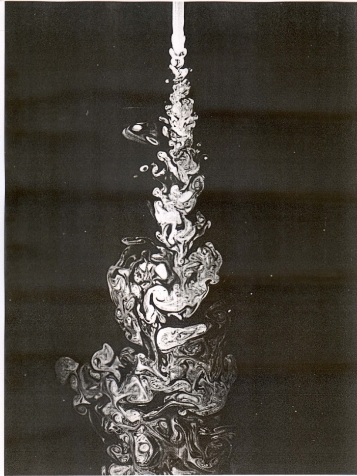
166. Turbulent water jet. Laser-induced fluorescence shows the concentration of jet fluid in the plane of symmetry of an axisymmetric jet of water directed downward into water. The Reynolds number is approximately 2300 .
