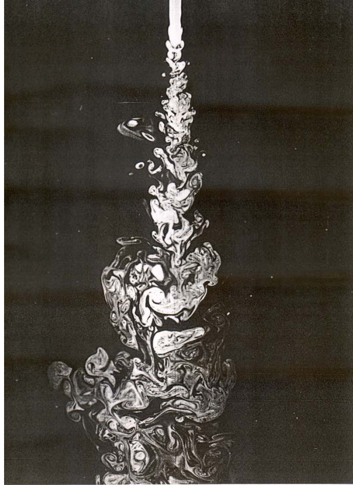
5. Turbulent water jet. Laser-induced fluorescence shows the concentration of jet fluid in the plane of symmetry of an axisymmetric jet of water directed downward to water. The Reynolds number is approximately 2300 .
