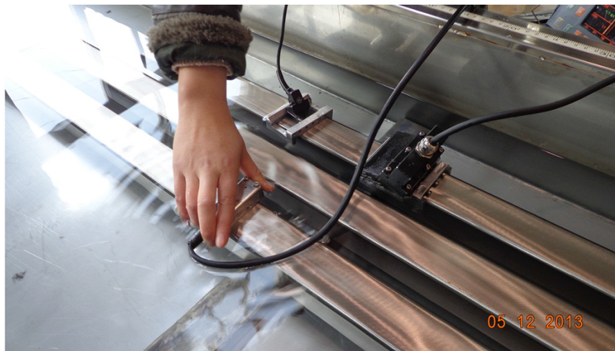
Figure 50. PAUT probes used at ASIPP for the NDE inspection of the PF2-5 jackets in water immersion (courtesy of J Qin, ASIPP).
