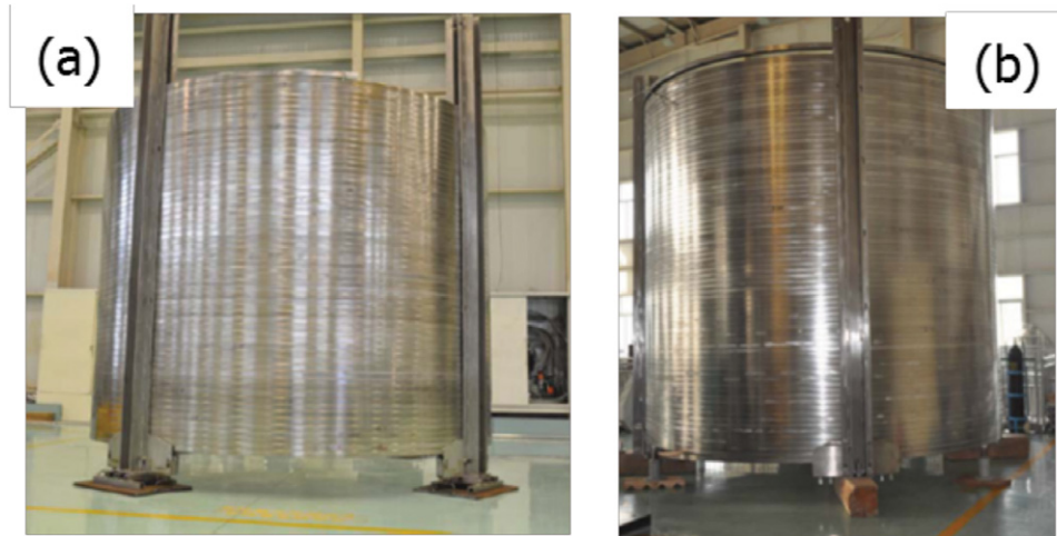
Figure 49. Views of first PF conductor ULs manufactured in China: (a) 740 m long Cu dummy UL and (b) 910 m long Cu dummy UL (courtesy of Y Wu, ASIPP).
