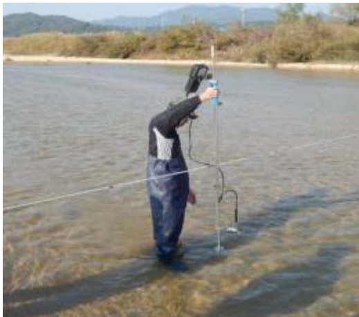
Velocity measurements with ADV
