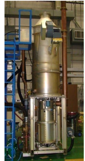
KSTAR ICRF wave generator: Transmitter (Tetrode tube)
