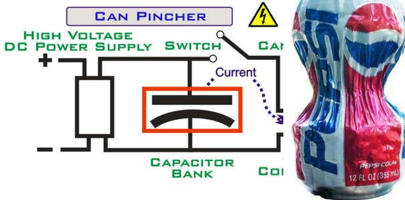
A theta pinch capable of crushing an aluminium soft drink can
