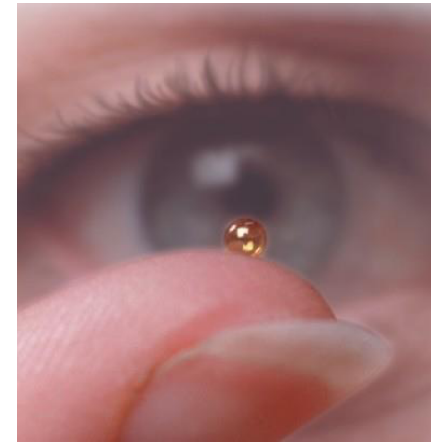
Image of an inertial confinement fusion fuel microcapsule. Taken from LLNL Sep. 2002 ST&R publication.
