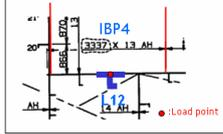
Design load acting on the longitudinals at inner bottom is equal to that on the inner bottom plate.
