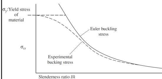
by theoretical consideration, a horizontal line of yield stress connected to Euler buckling stress is specified as an upper limit of Euler's buckling curve.
