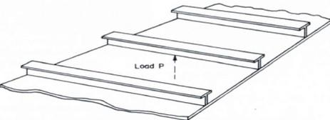
(a) Beams attached to plating
