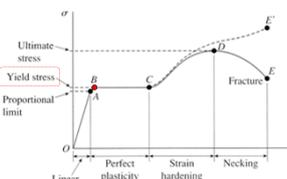
\* Yield Stress ( $\sigma_y$ ) [N/mm<sup>2</sup>] or [MPa]: The magnitude of the load required to cause yielding in the beam.<sup>2)</sup>
