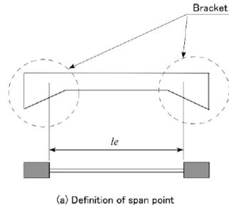
Ship structure members are usually connected with brackets or other structures.
