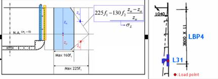
**②** ✓ Required Section Modulus    ✓ Allowable stress
