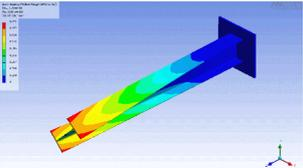
Torsional bending (1<sup>st</sup> mode)
