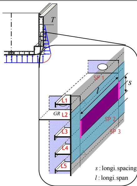
✓ The pressure at the load point is considered as **uniform load**
