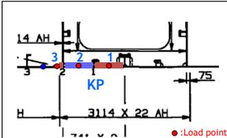
✓ Keel plate is composed of the three unit strips.
