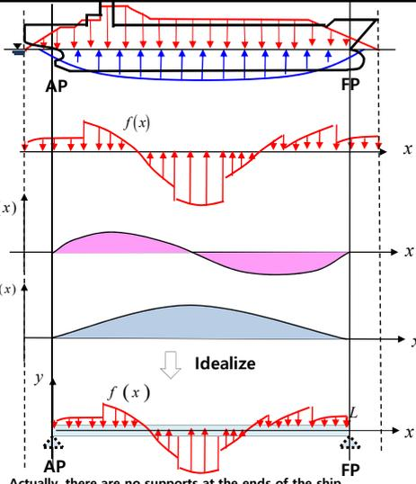
Actually, there are no supports at the ends of the ship. However, the deflection and slope could occur due to inequality of the buoyancy and the weight of a ship. For this problem, we assume that there are simple supports at the A.P and the F.P.
