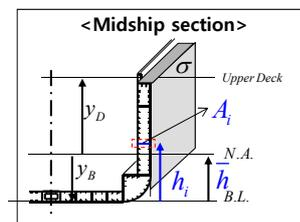
By definition, neutral axis pass through the centroid of the cross section.
