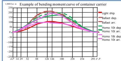
Example of bending moment curve of container carrier
