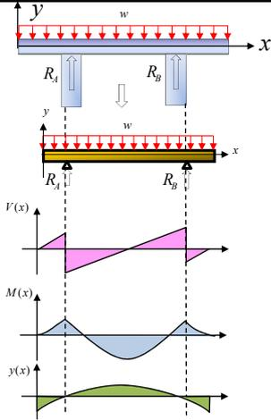
If there are supports at the ends, deflection and slope of the beam occur.
