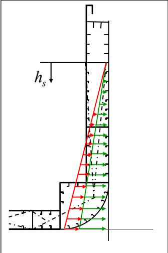
$$P_1 = \underbrace{\rho g_0 h_s}_{\text{Static Pressure}} + \underbrace{0.5 \rho a_v h_s}_{\text{Dynamic Pressure}}$$
