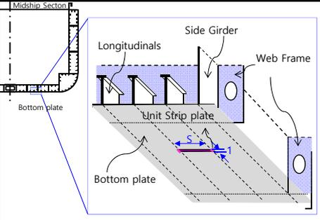
$P$  : "pressure" on the load point for the stiffener
