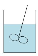
plug flow systems: no mixing in the direction of flow; homogeneous (completely mixed) in the direction perpendicular to the flow
