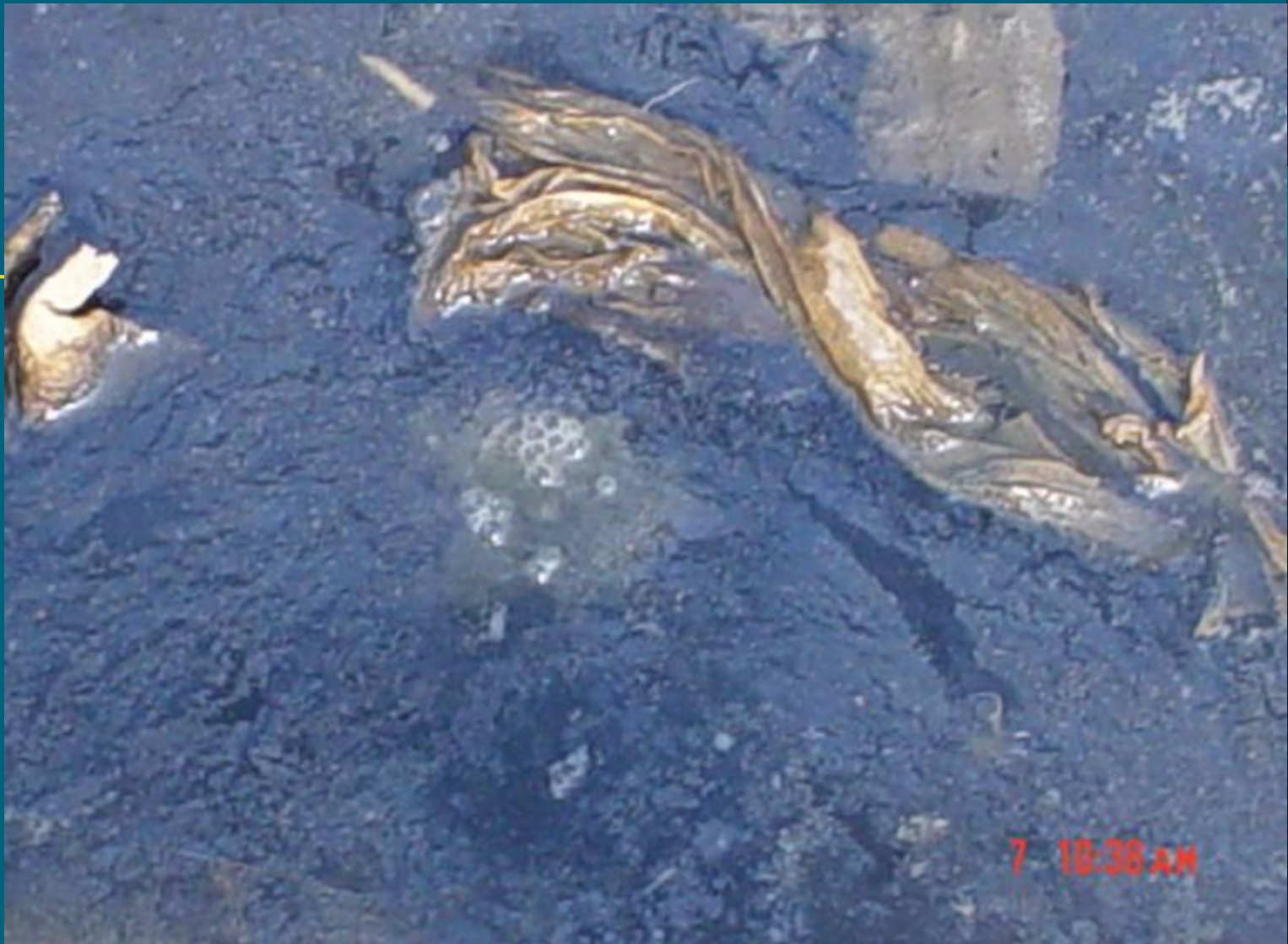
Leachate oozing out from covering soil
