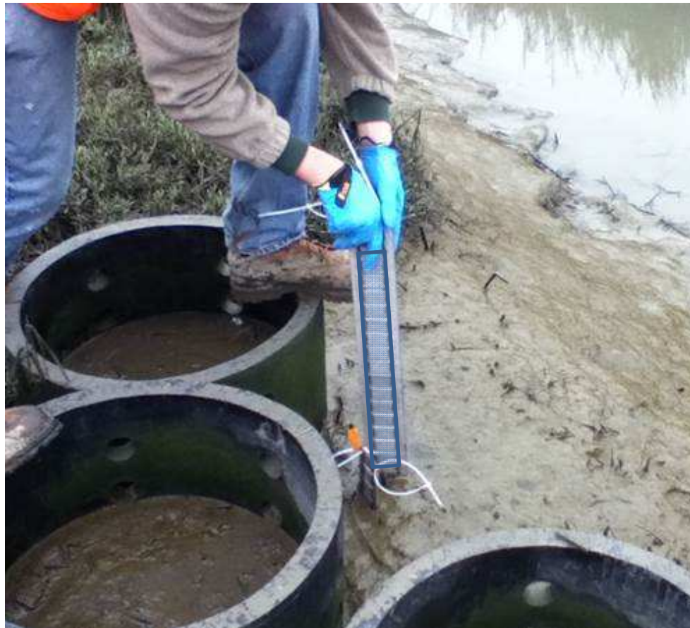
Measurement of depth-profile of sediment pore-water HOC concentrations in the field
