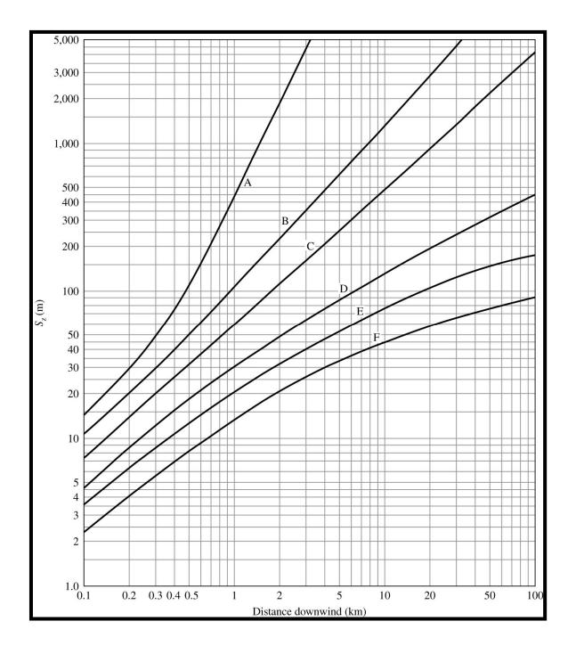
**Q:** A coal-fired power plants emits  $SO_2$  at a rate of 1656 g/s. At 3 km downwind on an overcast summer afternoon, what is the concentration of  $SO_2$  on the ground? The following parameters apply.
