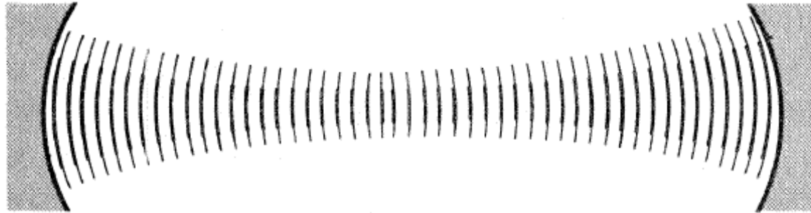
Figure 9.11. Standing wave pattern and lateral distribution of the TEM_{0,0} mode of a confocal laser cavity.
