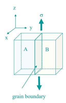
Because one grain has a **larger value of**  $\cos \phi \cos \lambda$  [smaller Taylor factor (1/m)], the above constraints restrict the deformation of this more favorably oriented grain and result in a *higher Yield Strength* (greater work-hardening response of the bicrystal.
