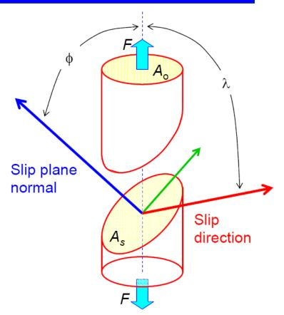
Plastic flow is initiated when  $\tau_{RSS}$  reaches a critical value, characteristic of the material, called *critical RSS*, when  $m \tau_{CRSS} = \sigma_{ys}$  (*Schmid law*).
