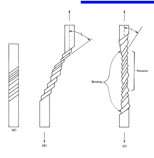
•Consider a single crystal oriented for slip on planes oriented  $\chi$  degrees from the tensile axis.
