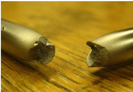
Fracture of tensile test specimen
