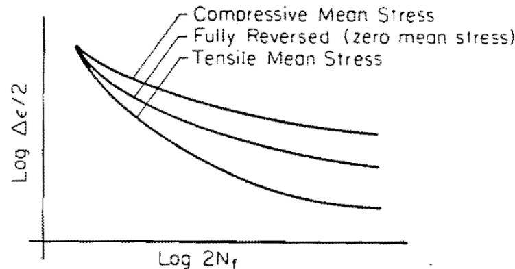
Figure 2.21\* Effect of mean stress on strain-life curve
