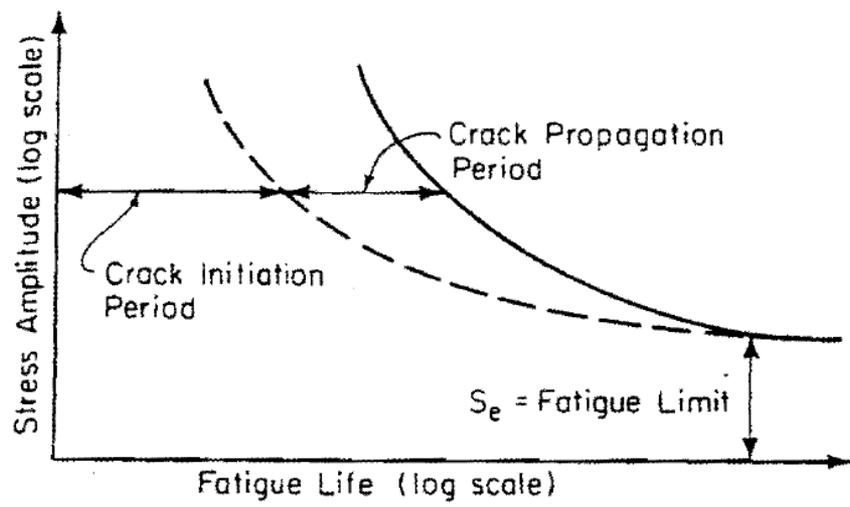
**Figure 3.1\*** Initiation and propagation portions of fatigue life
