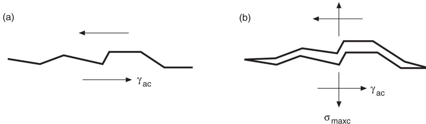
**Figure 14.14** Crack under pure shear (a), where irregularities retard growth, compared with a situation (b) where a normal stress acts to open the crack, enhancing its growth. (Adapted from [Socie 87]; used with permission of ASME.)
