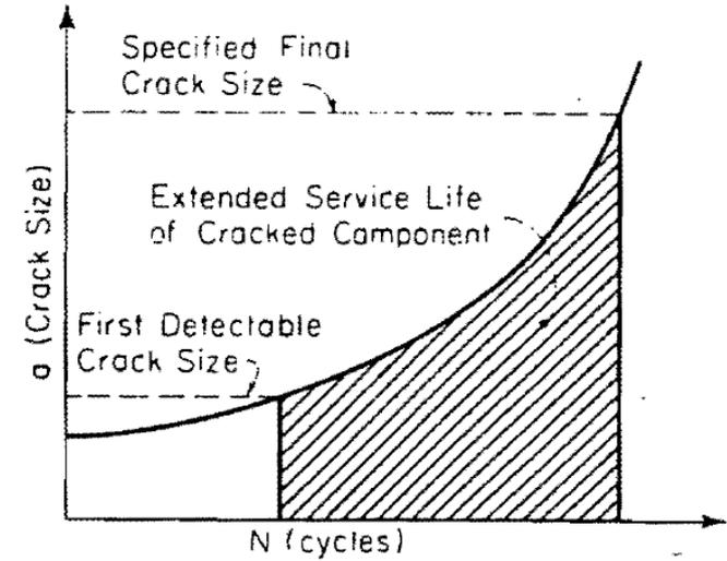
**Figure 3.9\*** Extended service life of a cracked component
