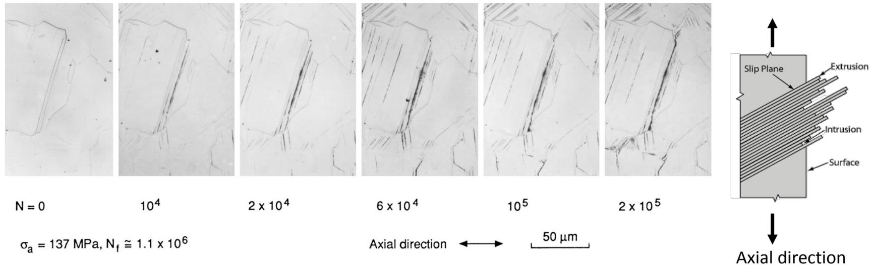
**Figure 9.17** The process of slip band damage during cyclic loading developing into a crack in an annealed 70Cu-30Zn brass.
