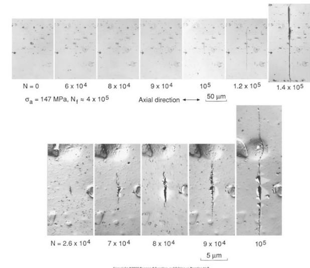
**Figure 1.8** Development of a fatigue crack during rotating bending of a precipitation-hardened aluminum alloy.
