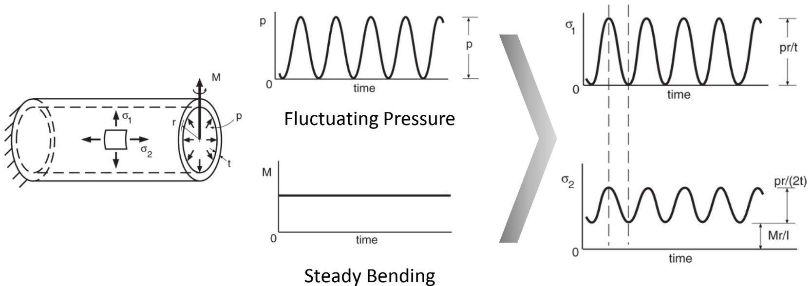
**Figure 9.40** Combined cyclic pressure and steady bending of a thin-walled tube with closed ends.
