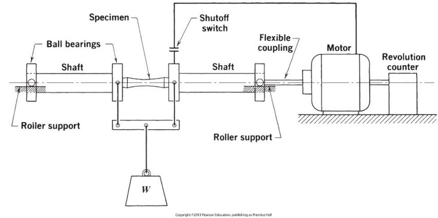
**Figure 9.11** Rotating cantilever beam fatigue testing machine used by **Wöhler**.
