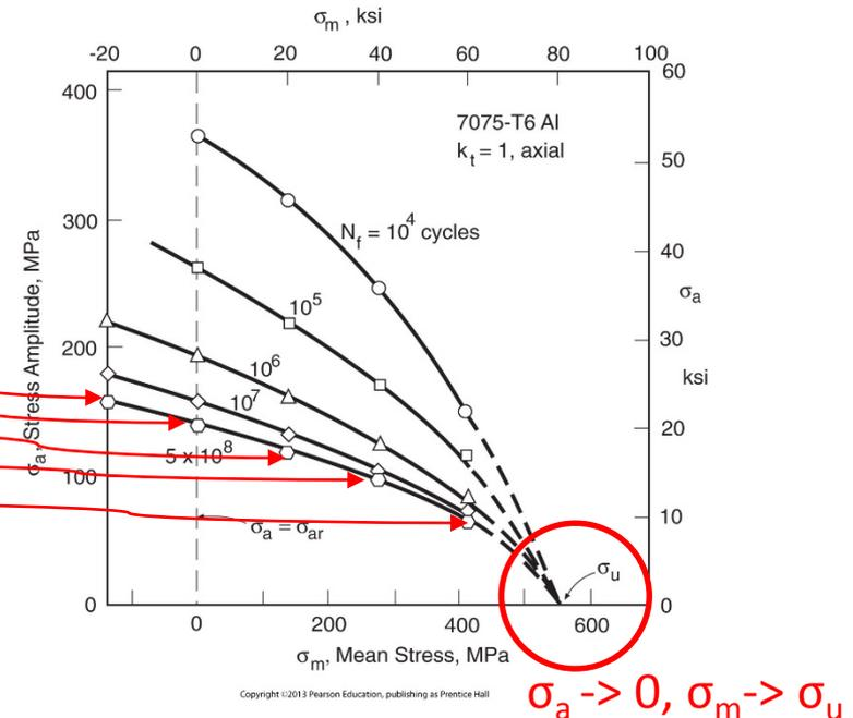
**Figure 9.37** Constant-life diagram taken from the S-N curves
