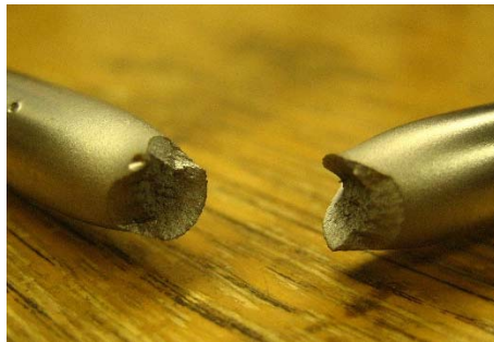
Fracture of tensile test specimen
