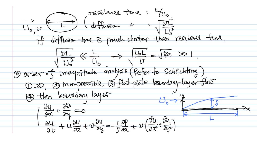
$$\left(\frac{\partial V}{\partial t} + U \frac{\partial V}{\partial x} + V \frac{\partial V}{\partial y} = -\frac{1}{9} \frac{\partial P}{\partial y} + V \left(\frac{\partial V}{\partial x} + \frac{\partial^2 V}{\partial y^2}\right)$$
