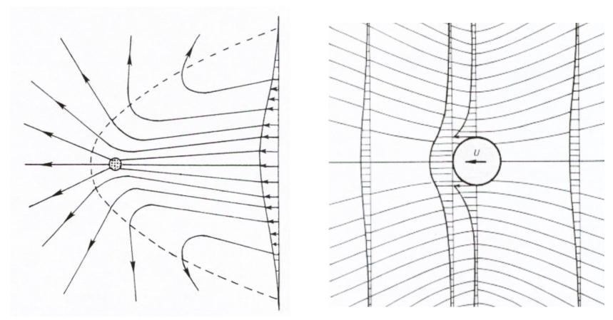
Note the upper stream and downstream asymmetry, a result of partial accounting for advection in the far field
