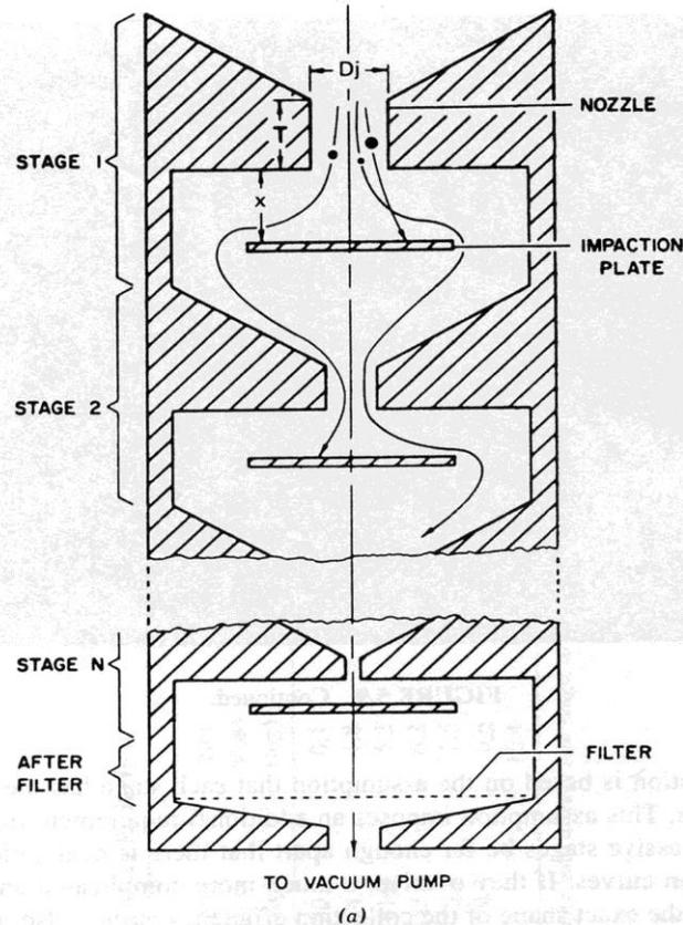
**FIGURE 5.9** Cascade impactor (a) Schematic diagram. Reprinted with permission from *Aerosol Measurement*, by Dale Lundgren et al. Copyright 1979 by the Board of Regents of the State of Florida. (b) Eight stage Anderson ambient cascade impactor with nozzle plate and impaction plate shown at left.
