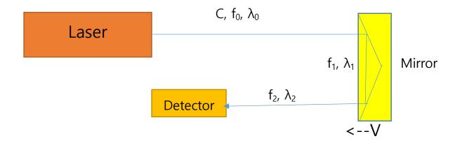
Let C be the speed of light, V be the velocity of mirror. When  $f_0$  is the frequency from laser source,  $f_1$  is the frequency observed at the mirror or corner cube, and  $f_2$  is the frequency measured at the detector.
