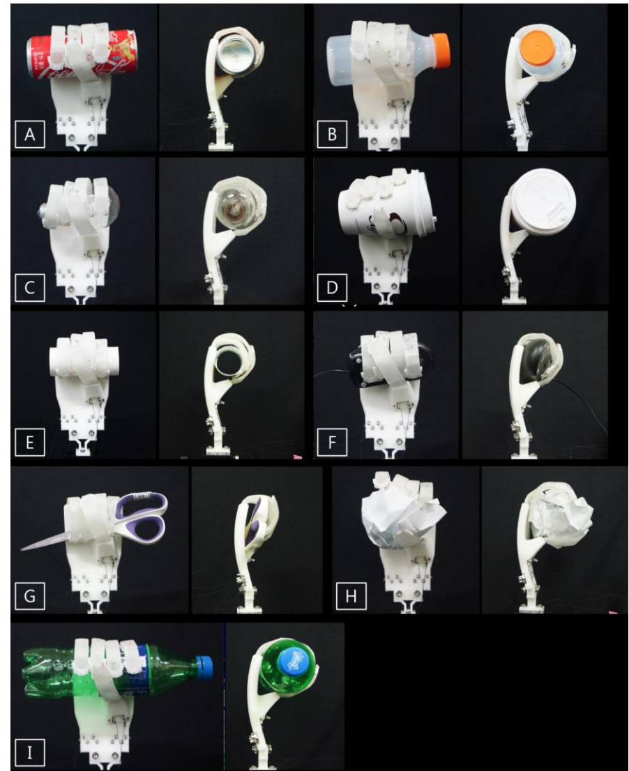
Sequences of images showing the bending actuation of the soft robotic hand prototype with a current of 0.8 A
