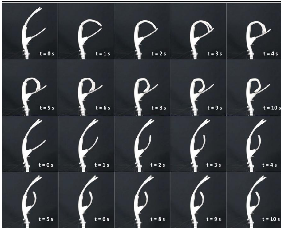
Sequences of images showing the bending actuation of the soft robotic hand prototype with a current of 0.8 A
