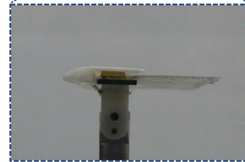
Wind tunnel test of soft morphing spoiler
