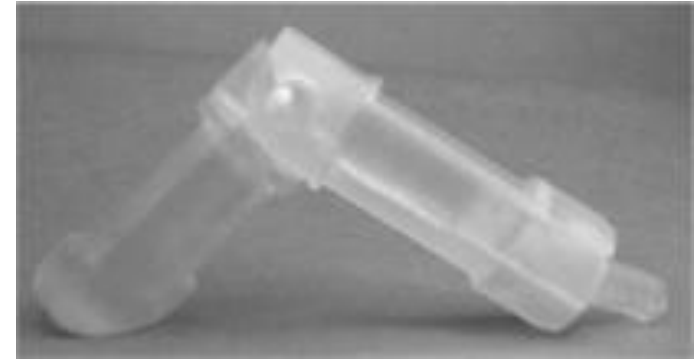
Robotic thumb built with SL (Stereolithography)
