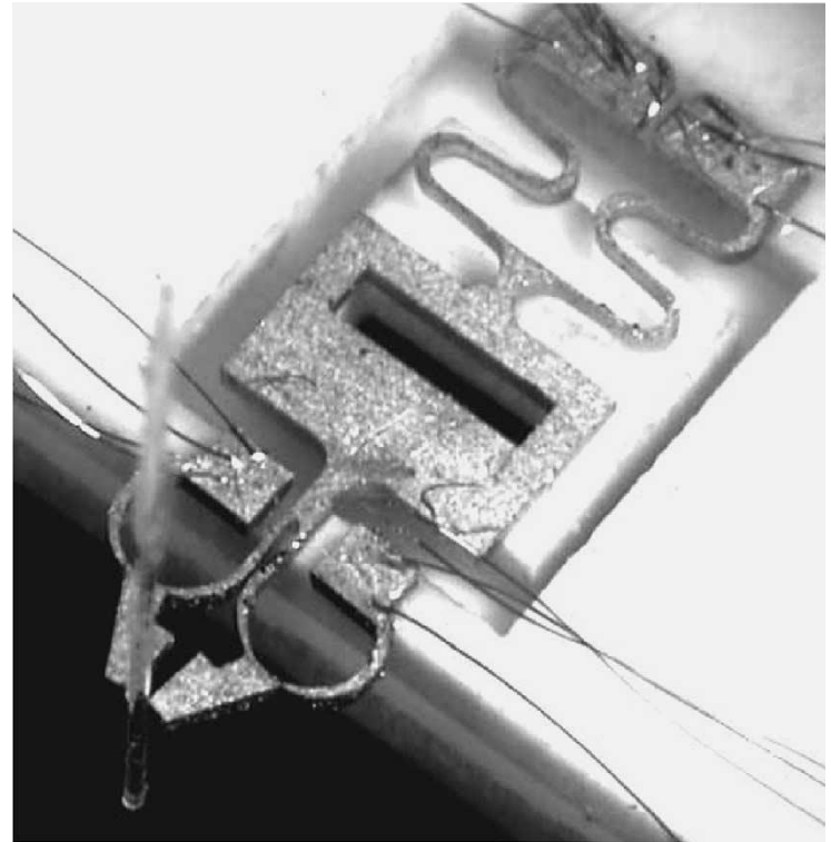
SMA micro gripper system holding a piece of optical fiber of 140 \mu\text{m} diameter
