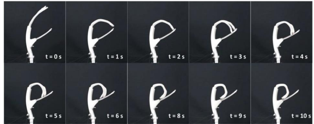
Sequences of images showing the bending actuation of the soft robotic hand prototype with a current of 0.8 A
