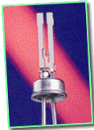
Tuning fork quartz resonator
