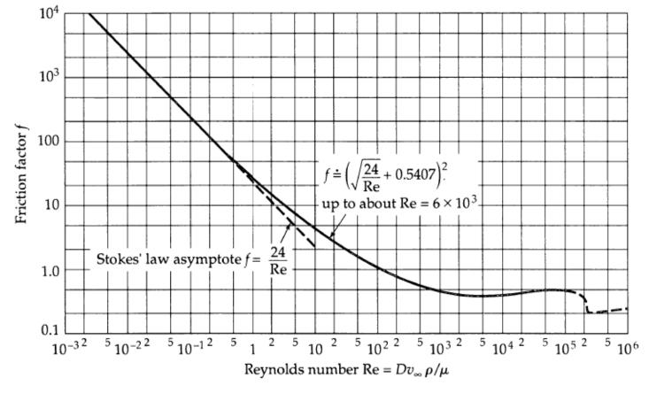
"Transport Phenomena" 2nd ed., R.B. Bird, W.E. Stewart, E.N. Lightfoot Friction factors for flow around spheres
