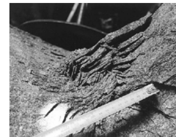
Fracturing at the tip of V-notch (Chandler, 2004)
