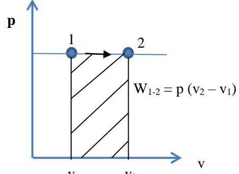
.05 kg heated at 2 bar until  $V_2 = .0658 \text{ m}^3$
