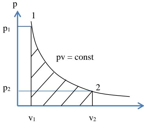
$$p_1 V_1 = p_2 V_2 = C$$
