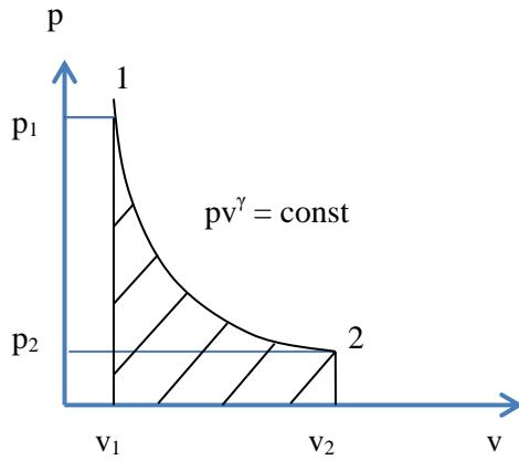
$$\begin{aligned} W &= \int_1^2 pdv = \int_1^2 \frac{Cdv}{V^\gamma} = C \left[ \frac{V^{1-\gamma}}{1-\gamma} \right]_{v_1}^{v_2} \\ &= C \frac{V_2^{1-\gamma} - V_1^{1-\gamma}}{1-\gamma} = C \frac{V_1^{1-\gamma} - V_2^{1-\gamma}}{\gamma-1} \\ &= \frac{p_1 V_1^2 V_1^{1-\gamma} - p_2 V_2^2 V_2^{1-\gamma}}{\gamma-1} \quad (C = p_1 V_1^\gamma = p_2 V_2^\gamma) \\ \therefore W &= \frac{p_1 V_1 - p_2 V_2}{\gamma-1} \end{aligned}$$
