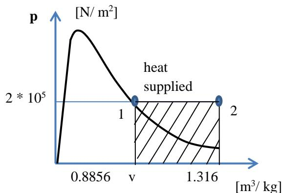
$$h_1 = h_g = 2707 \text{ kJ/kg at 2 bar}$$
