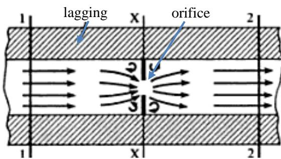
$$h_1 + \frac{V_1^2}{2} + q = h_2 + \frac{V_2^2}{2} + w$$
