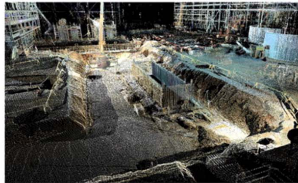
b) Registered point cloud of laser scans
