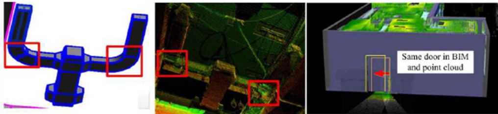
a. an example showing shape discrepancy in the air duct section analyzed in the case
