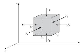
pressure forces acting on a static fluid element
