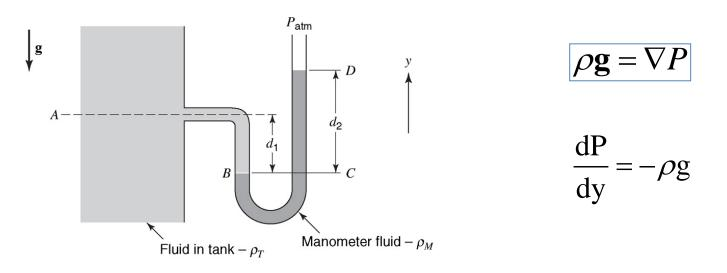
integrating between C and D in manometer fluid
